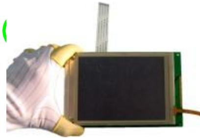
As above picture, please handle with anti-static gloves around LCM edges.
