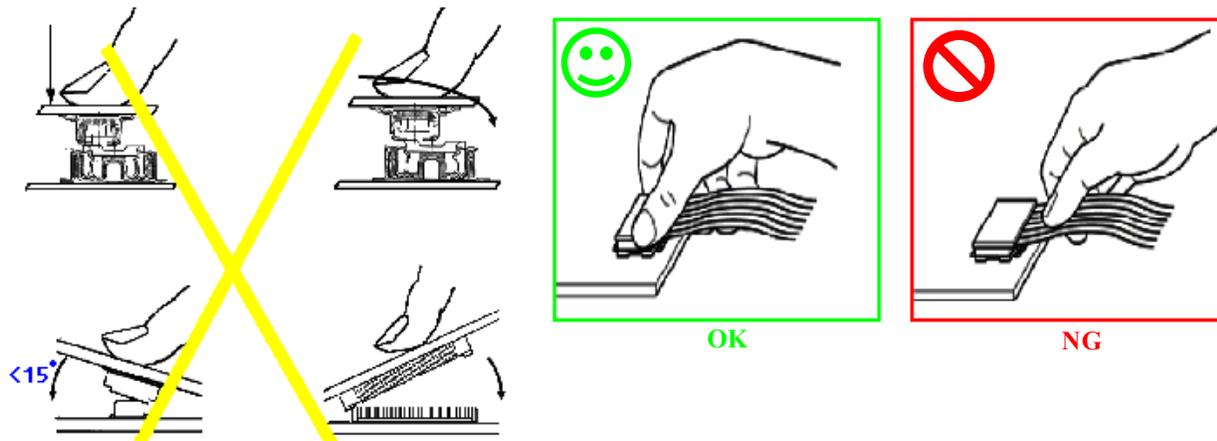
**Precaution for soldering the LCM**
